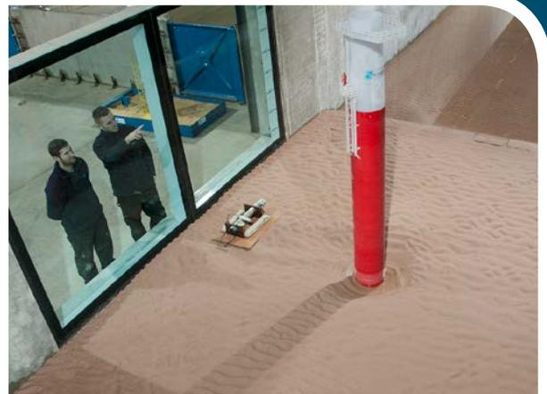
The Fast Flow Facility is one of the world's largest marine test facilities. This dual-channel, race track shaped flume is a unique large scale modelling facility offering wave, fast tidal current and sediment capabilities.
