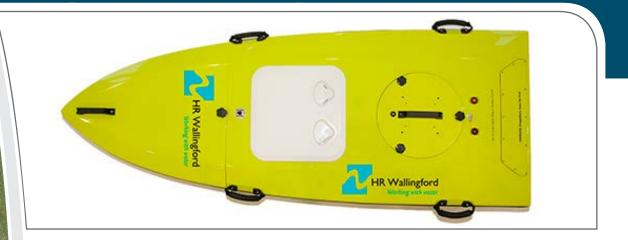
The ARCboat is a remote controlled boat that is used to collect river and estuarine data including flow, depth and suspended sediment concentrations.
